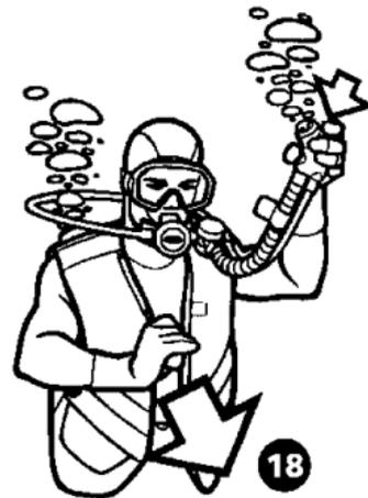
**C > Lower exhaust valve:** found at the back on the lower right-hand side of the BC.
